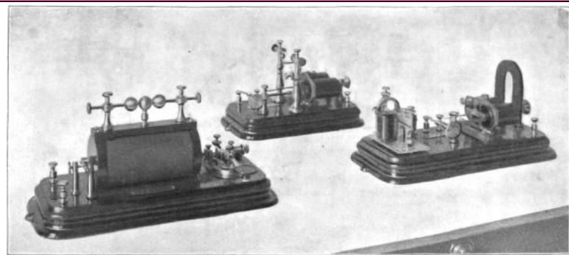
INSTRUMENTS FOR TRANSMITTING MORSE SIGNALS BY MEANS OF WIRELESS TELEGRAPHY.
